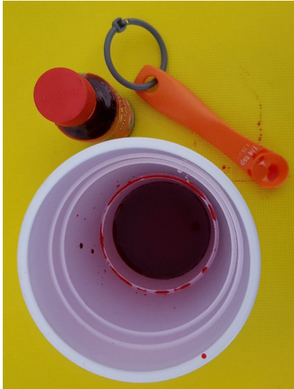
Required volume of water placed in cup, teaspoon used to measure dye and place in cup.
