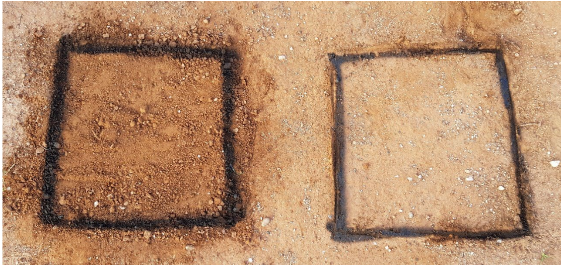
Treatments marked out, treatment 2 (left) has been implemented. A channel was dug on the down side of the treatments to allow a jar to easily collect run off water.
